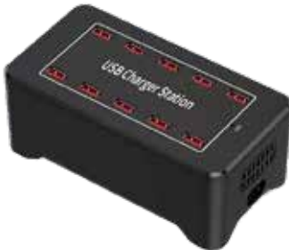
No. MC001 10-port charger Total current 20A Total power 100W USB single port output 2.4A (MAX) 25-35-00
